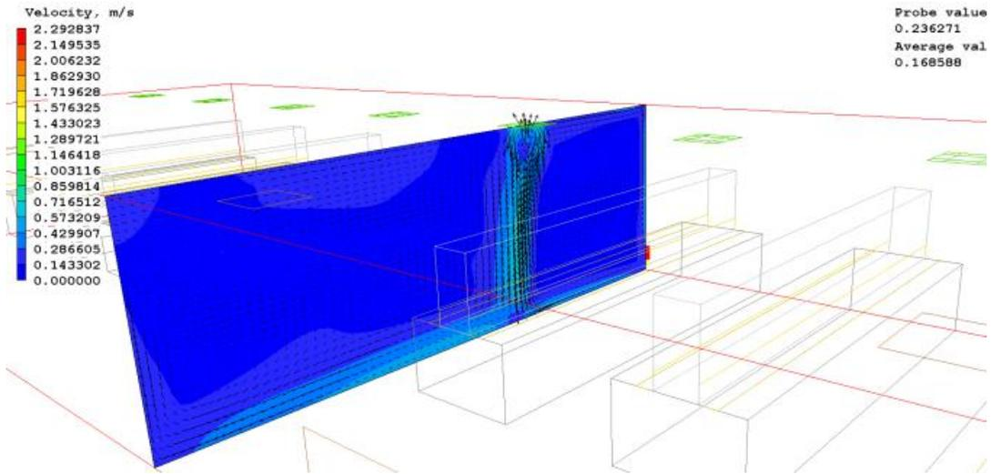
Figure-35 VAV System Velocity Profile Overview in X-direction
