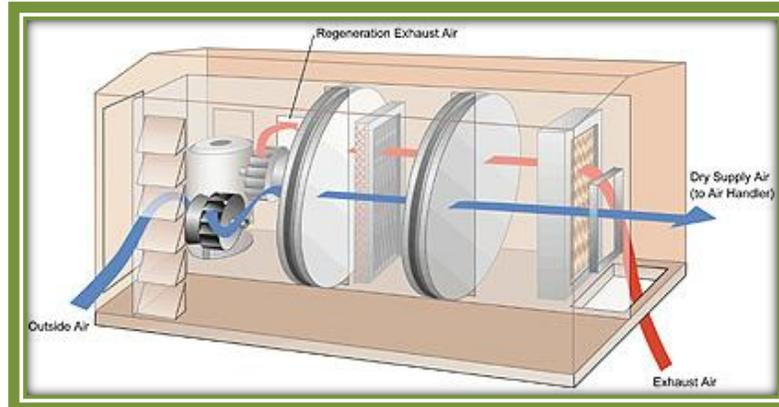
**Figure-17** Heat Recovery System – Enthalpy Wheel
