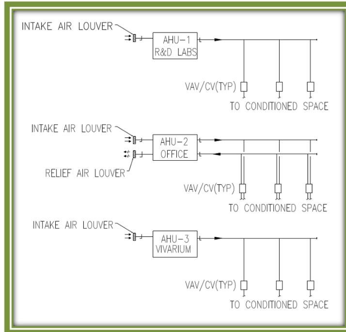
**Figure-5** Air Side Schematic
