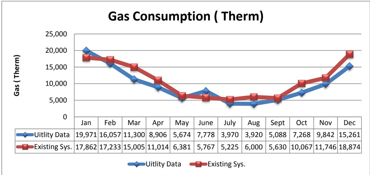
**Figure-12** Gas Consumption Comparison between Model and Utility Data
