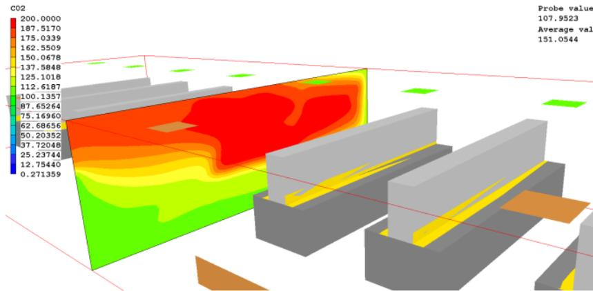
**Figure-44** VAV System Contaminant Profile Overview in X-direction at the Edge of the Bench
