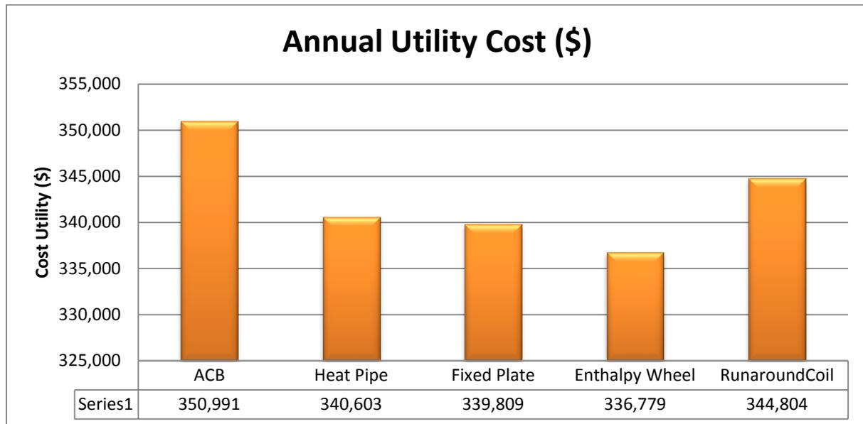
**Figure-54** Heat Recovery Systems Annual Utility Cost Comparison
