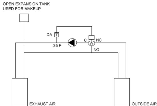
**Figure-55** Runaround Coil System Control Schematic
