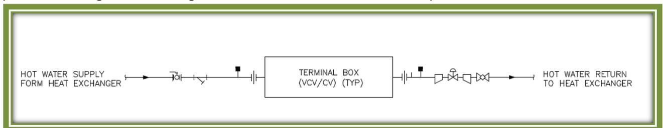
**Figure-7** Water Side Hot Water Schematic
