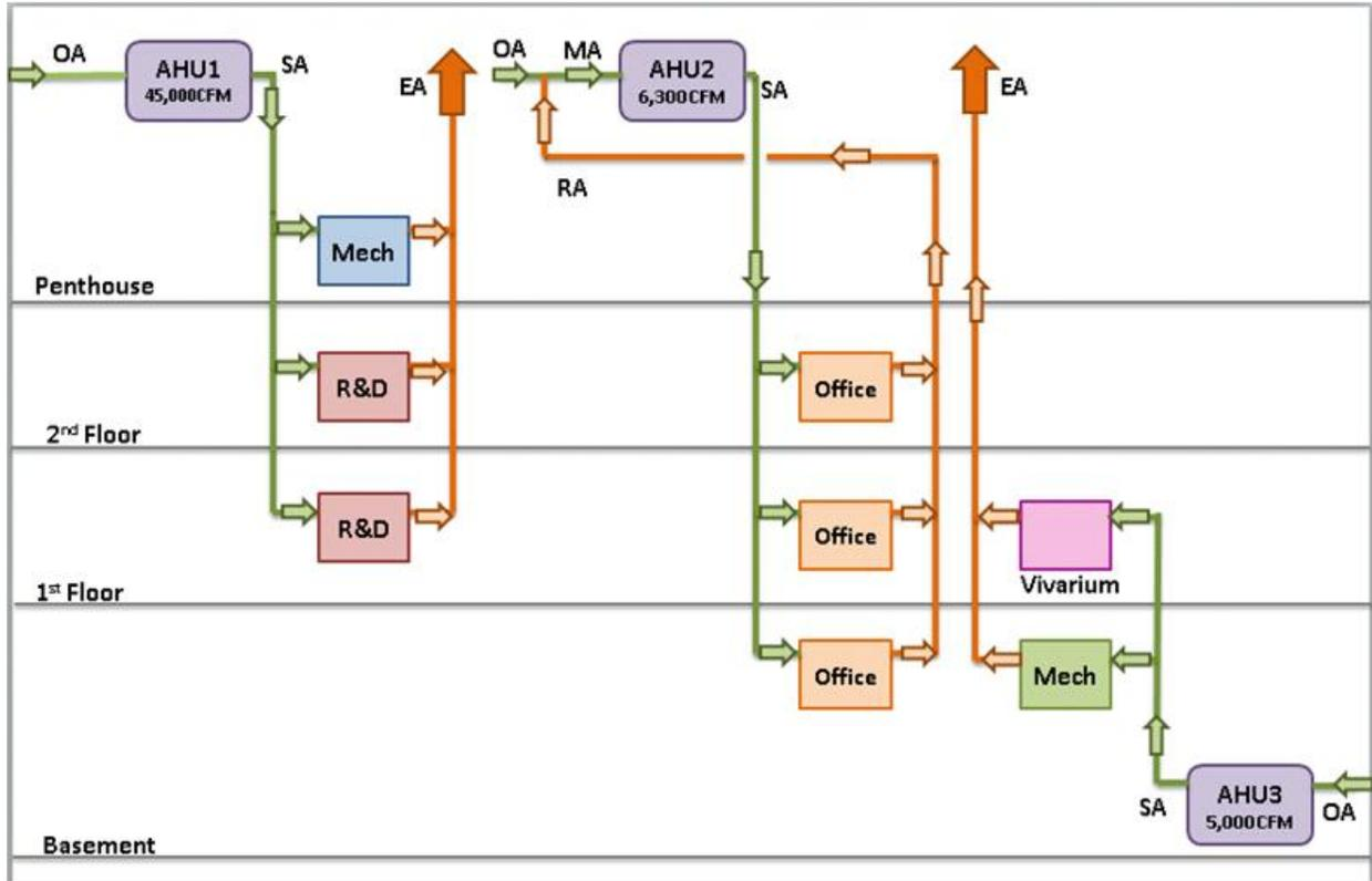
Figure-23 Active Chilled Beam Air Side Riser Diagram
