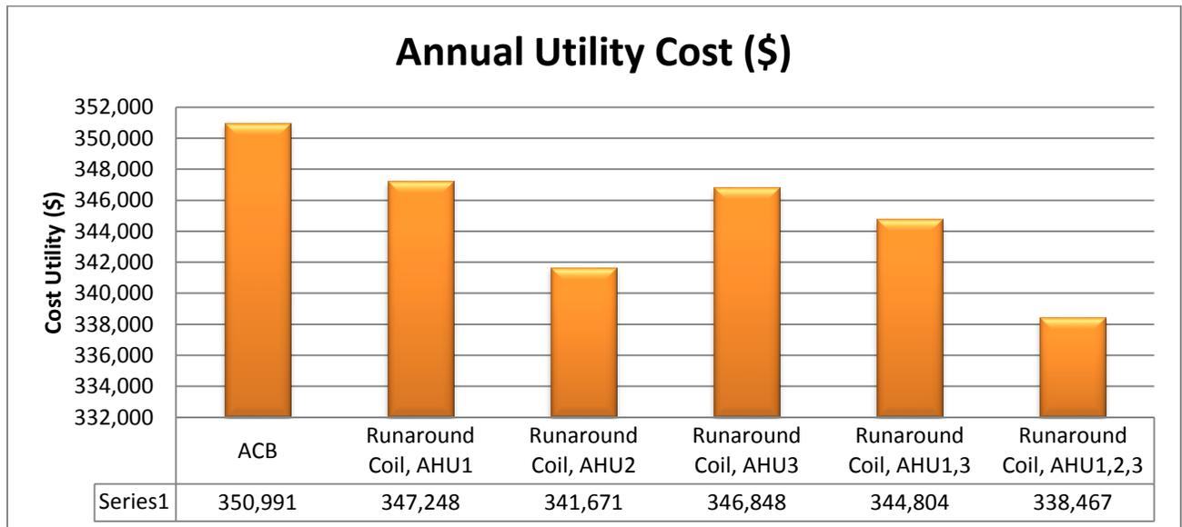
Figure-59 Runaround Coil System Annual Utility Cost Comparison
