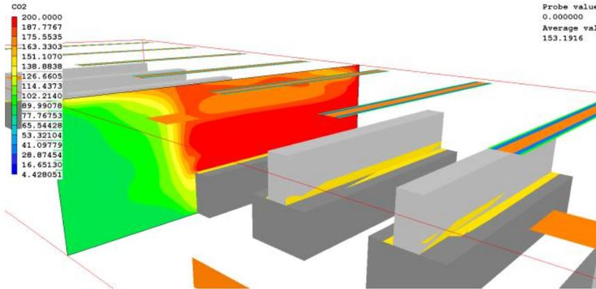
Figure-46 ACB System Contaminant Profile Overview in X-direction at the Source
