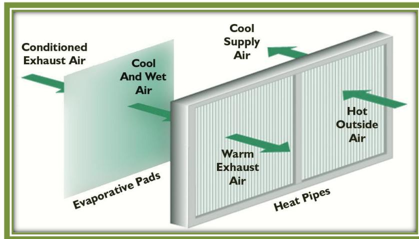
Figure-19 Heat Recovery System – Heat Pipe
