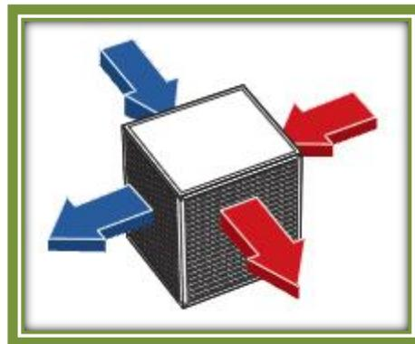
**Figure-18** Heat Recovery System – Fixed Plate Heat Exchanger
