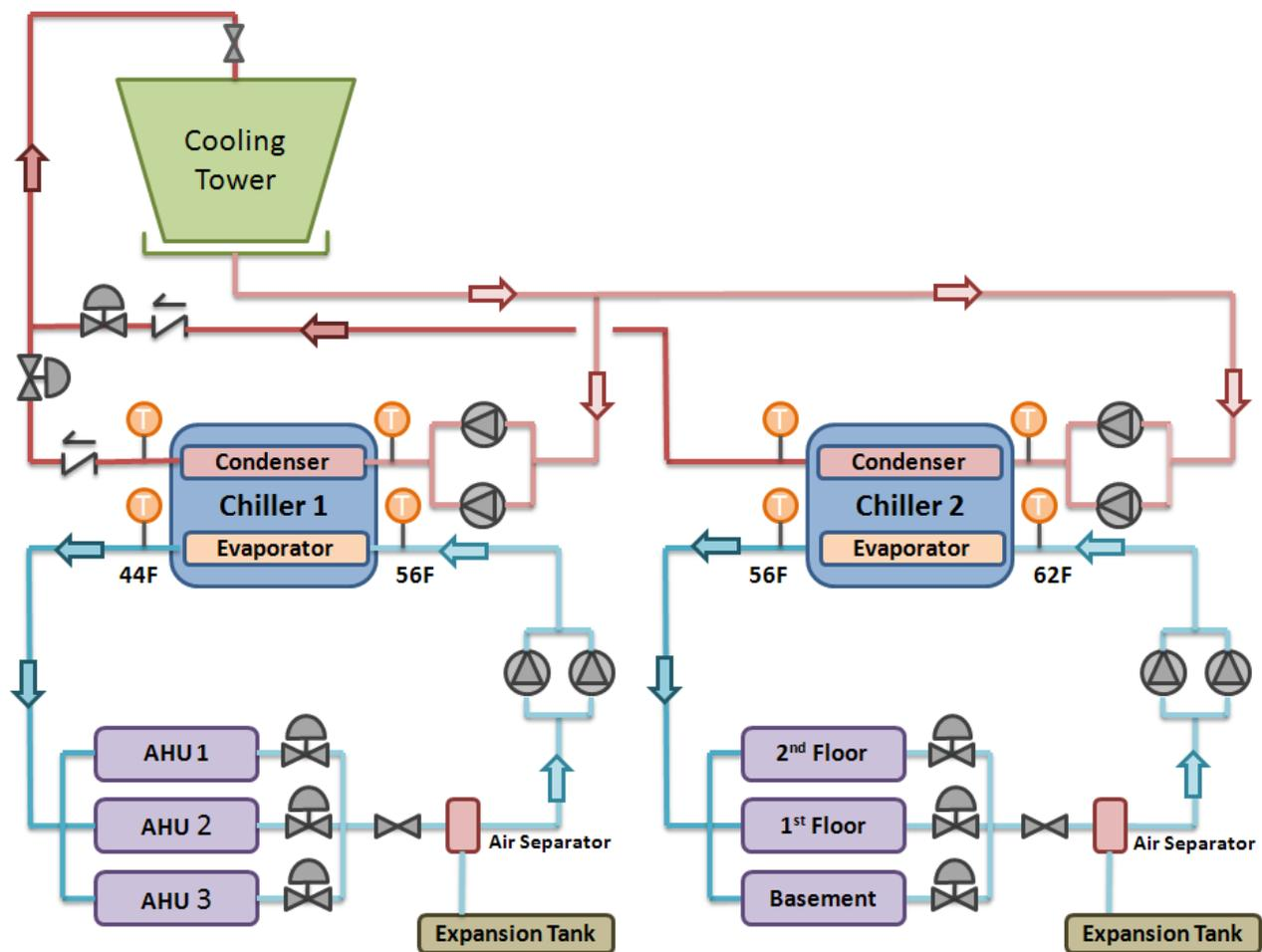
Figure-22 Active Chilled Beam Water Side Cooling Schematic
