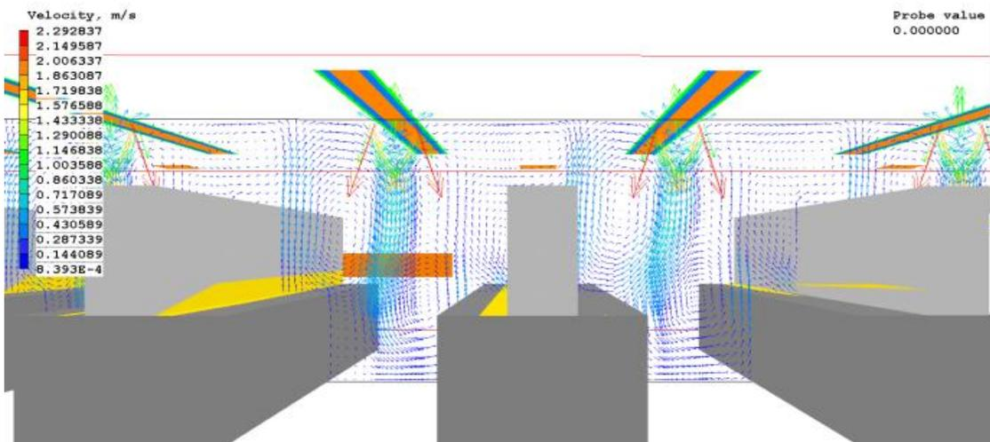
Figure-34 ACB System Velocity Profile Close View in Y-direction
