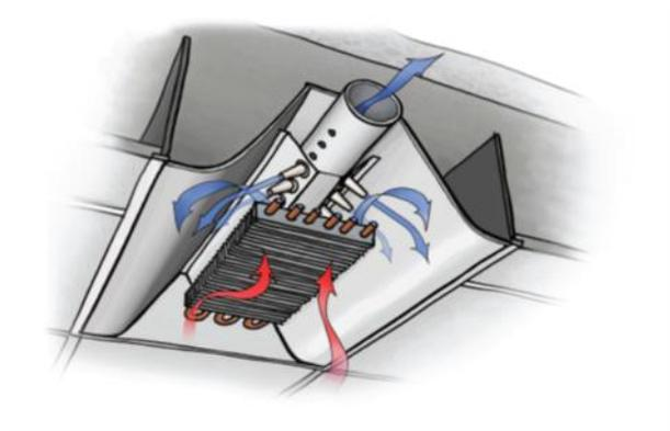
**Figure-16** Active chilled beam systems use air supplied from an air handling unit
