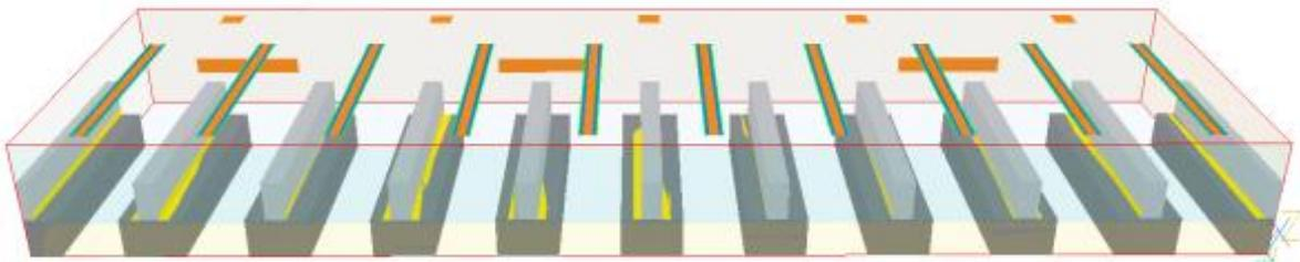
Figure-28 Active Chilled Beam Layout – Elevated View
