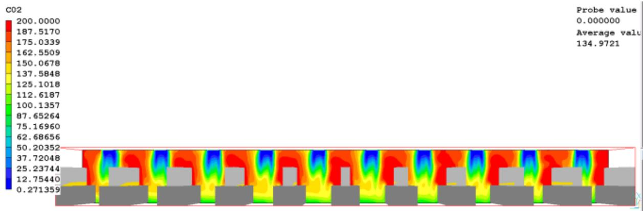
Figure-41 VAV System Contaminant Profile Overview in Y-direction
