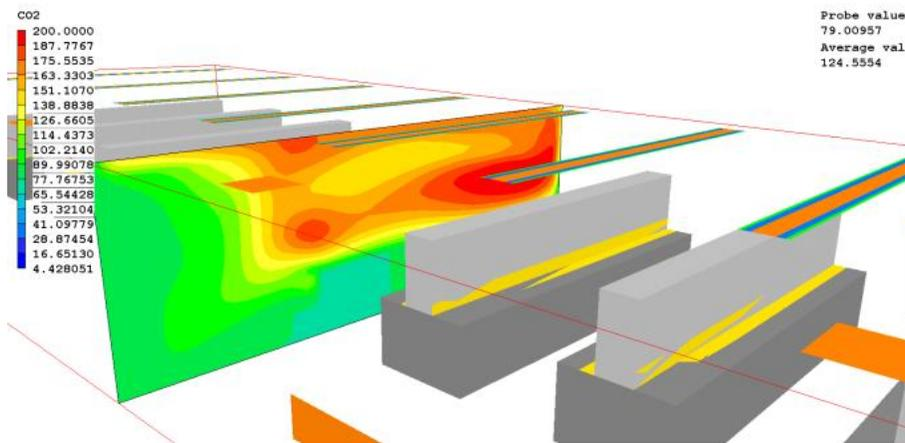
Figure-47 ACB System Contaminant Profile Overview in X-direction at the Edge of the Bench
