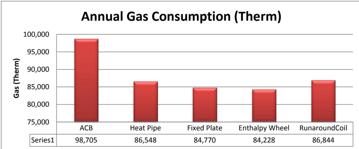
Figure-53 Heat Recovery Systems Annual Gas Consumption Comparison
