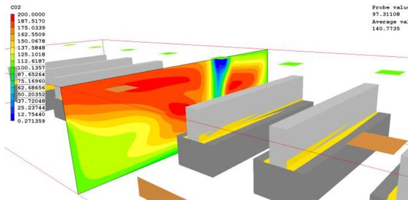
**Figure-45** VAV System Contaminant Profile Overview in X-direction in the Walkway between Benches
