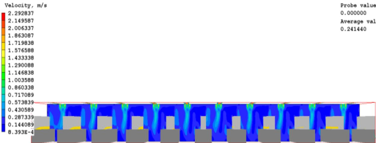
Figure-32 ACB System Velocity Profile Overview in Y-direction
