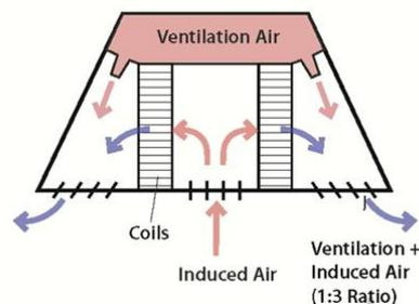
Figure-21 Active Chilled Beam Section
