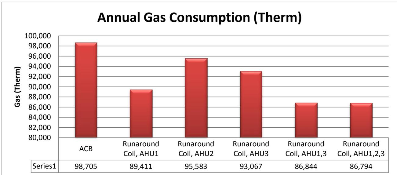
**Figure-58** Runaround Coil System Annual Gas Consumption Comparison
