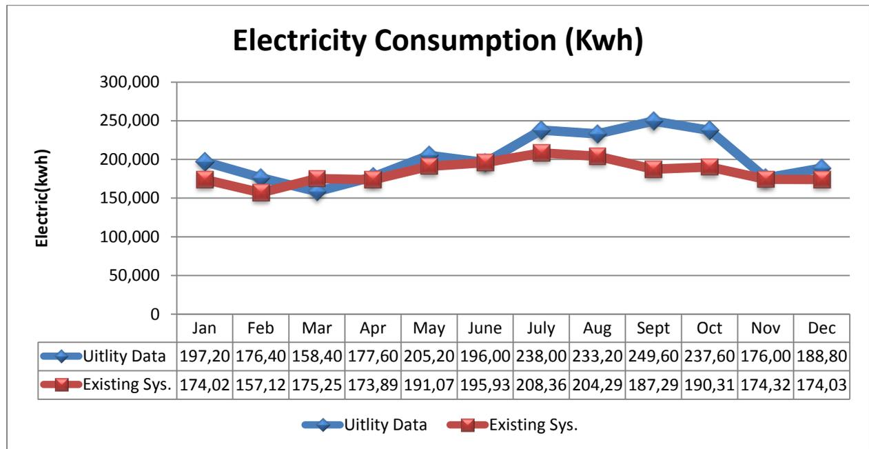
**Figure-11** Electricity Consumption Comparison between Model and Utility Data
