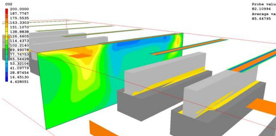
Figure-48 ACB System Contaminant Profile Overview in X-direction in the Walkway between Benches
