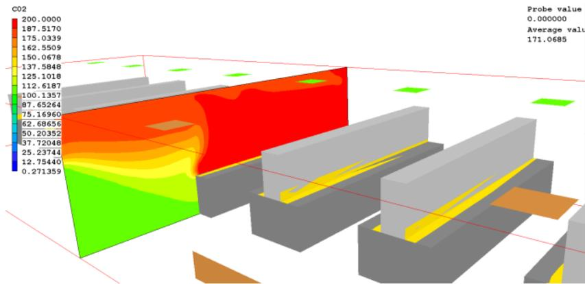
**Figure-43** VAV System Contaminant Profile Overview in X-direction at the Source
