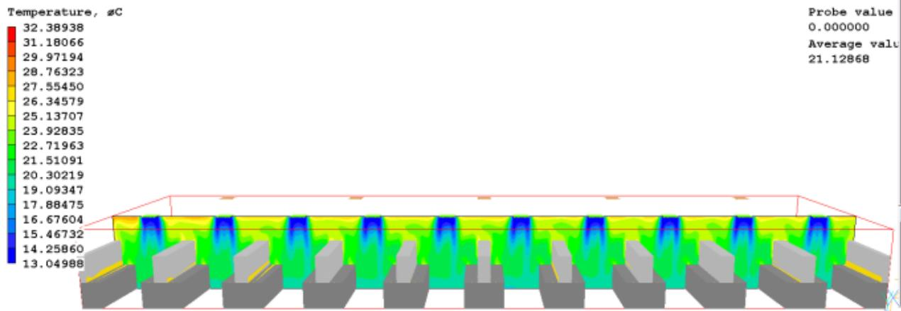
Figure-37 VAV System Temperature Profile Overview in Y-direction
