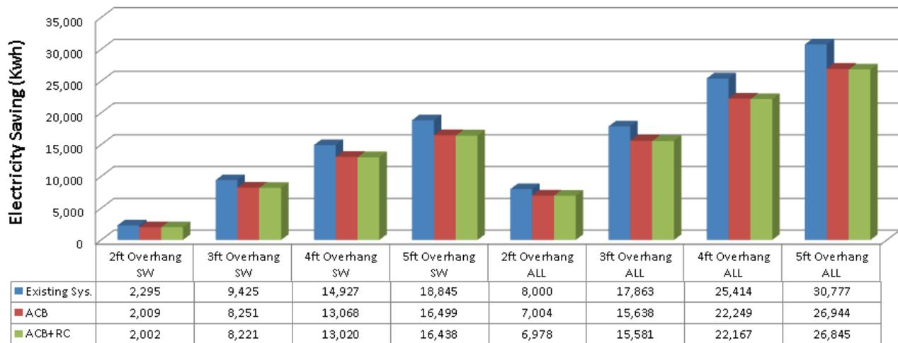
**Figure-71 Solar Shading System Electricity Consumption Saving**
