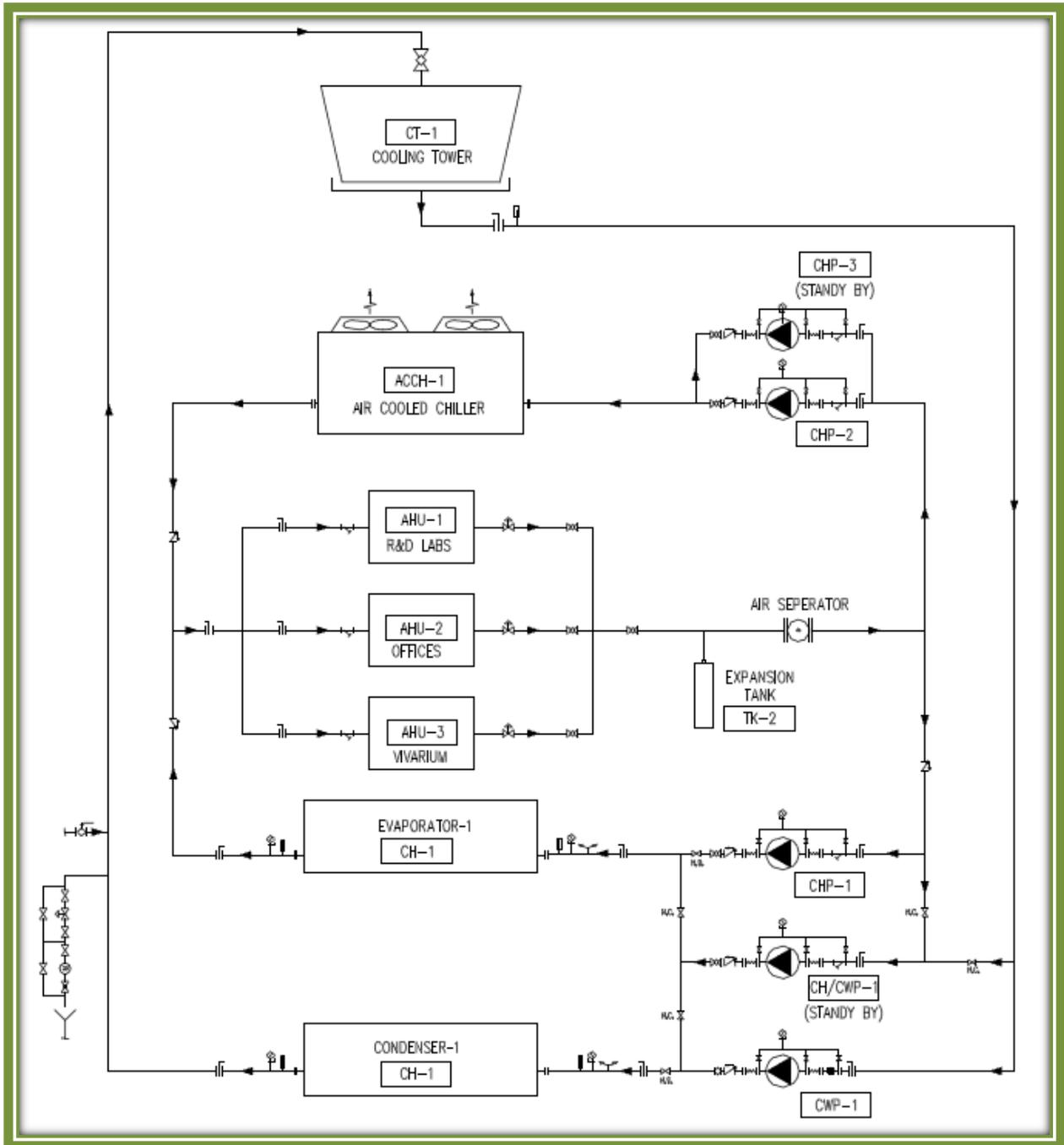
Figure-6 Water Side Cooling Schematic
