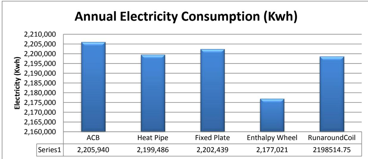
Figure-52 Heat Recovery Systems Annual Electricity Consumption Comparison
