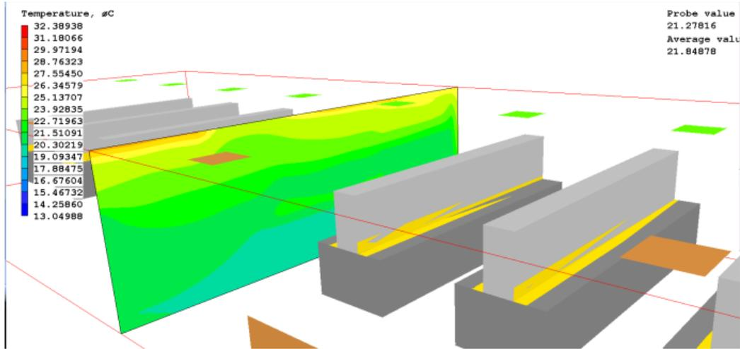
Figure-39 VAV System Temperature Profile Overview in X-direction
