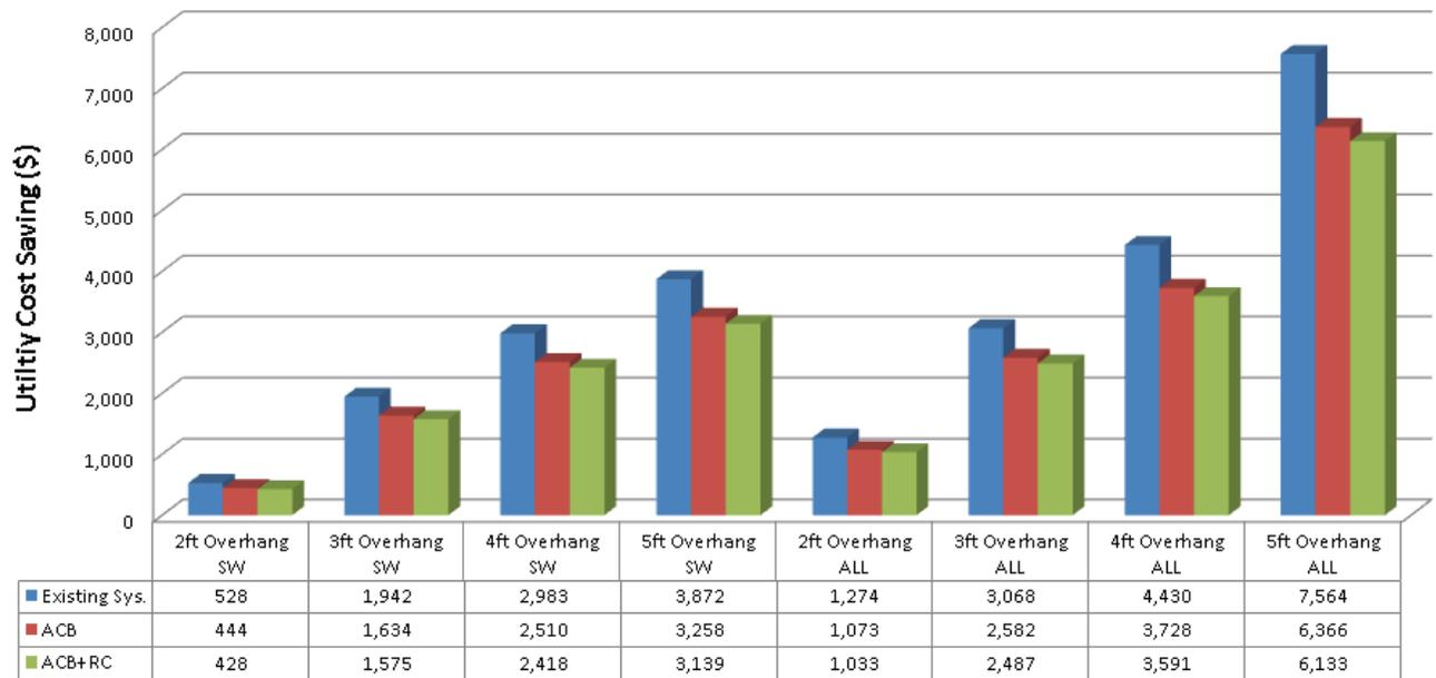
Figure-73 Solar Shading System Utility Cost Saving
