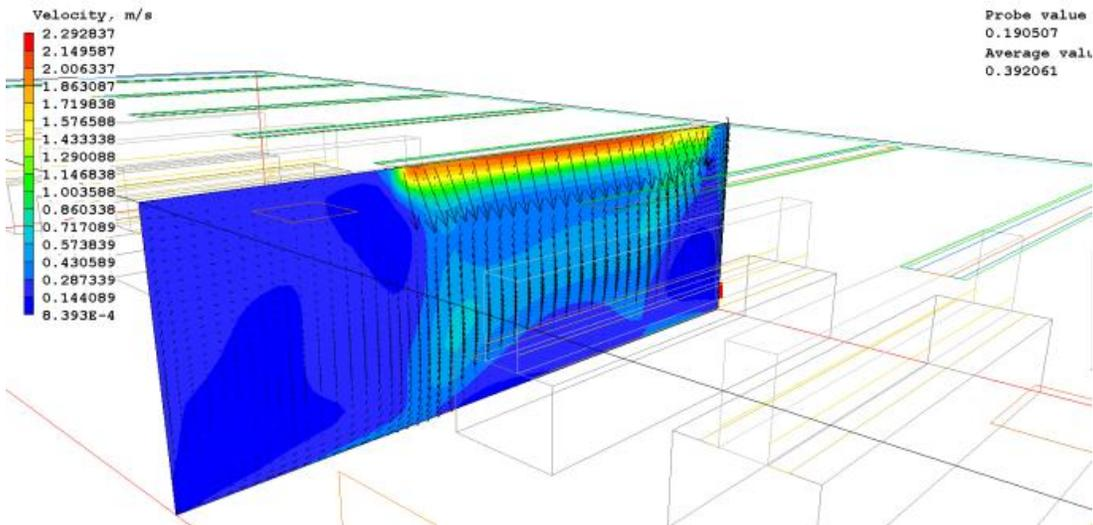
Figure-36 ACB System Velocity Profile Overview in X-direction
