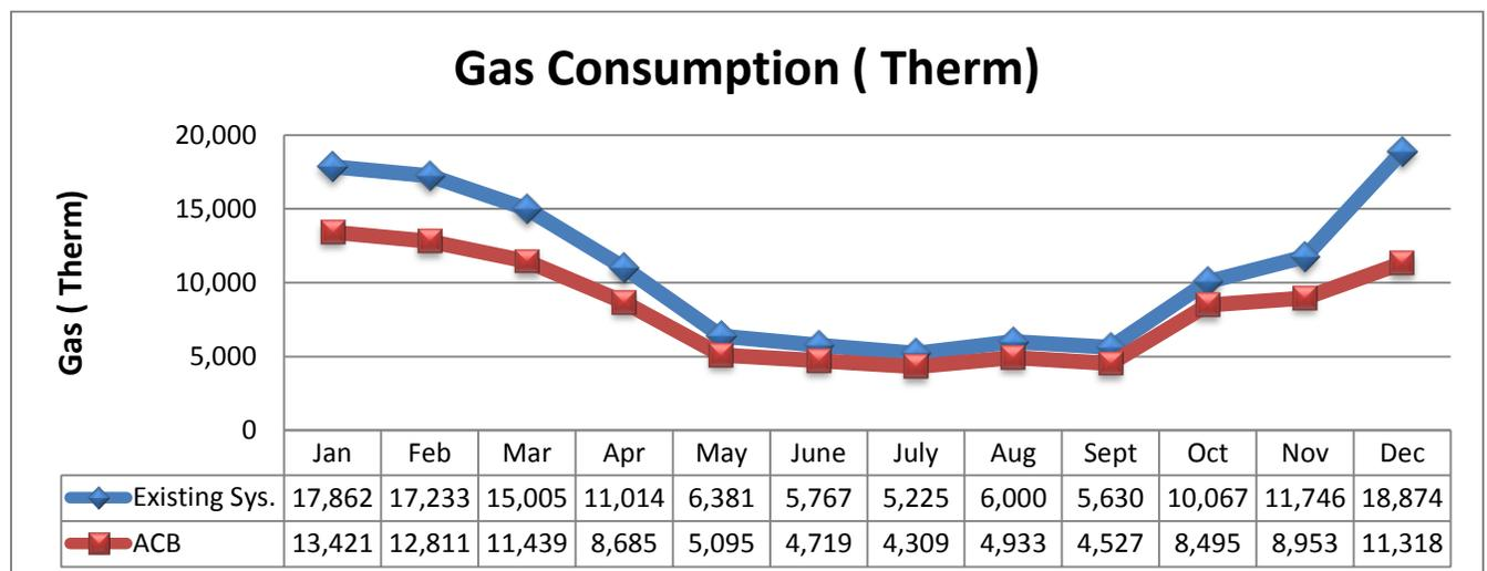
Figure-50 Gas Consumption Comparison
