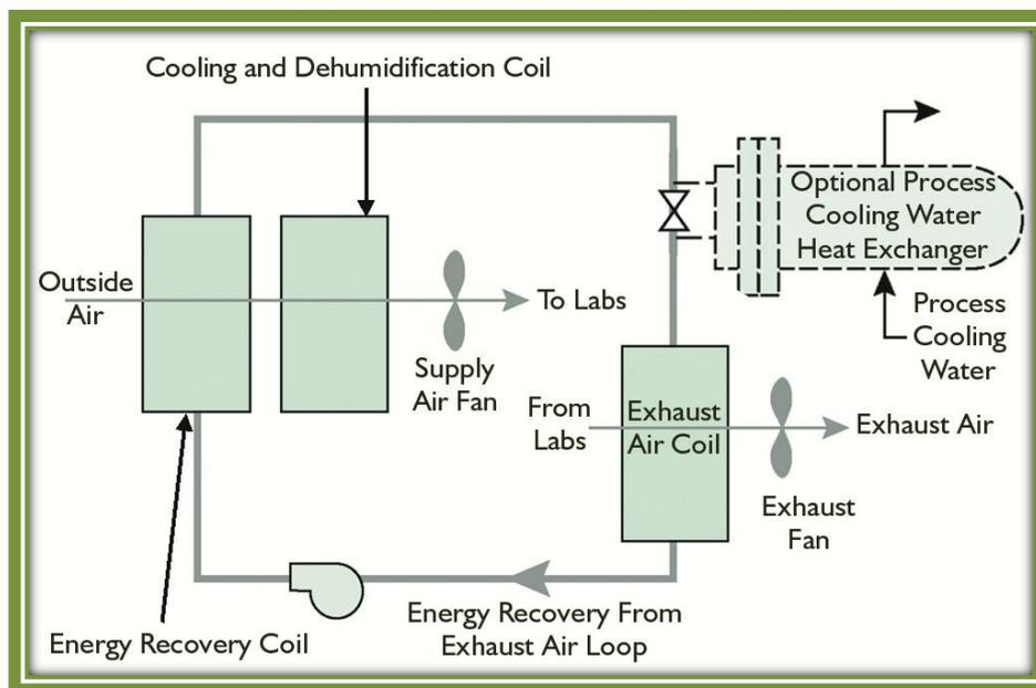
Figure-20 Heat Recovery System – Runaround Loop
