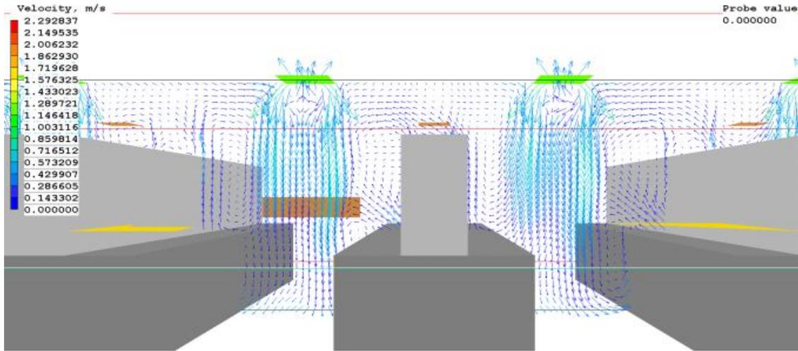
Figure-33 VAV System Velocity Profile Close View in Y-direction
