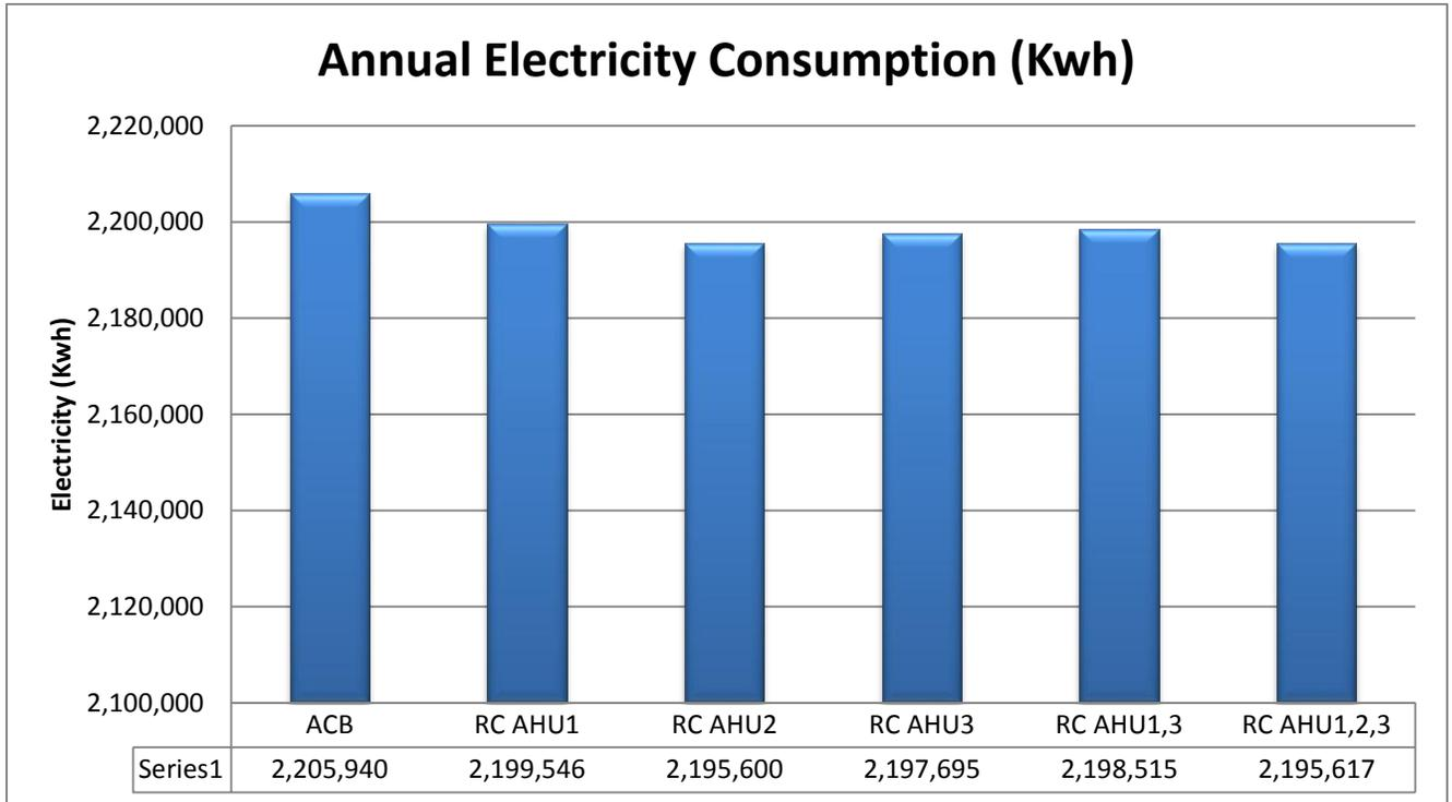
**Figure-57** Runaround Coil System Annual Electricity Consumption Comparison
