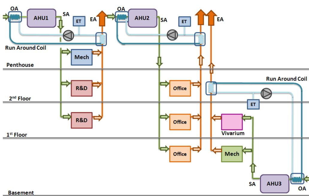
Figure-56 Runaround Coil System Schematic
